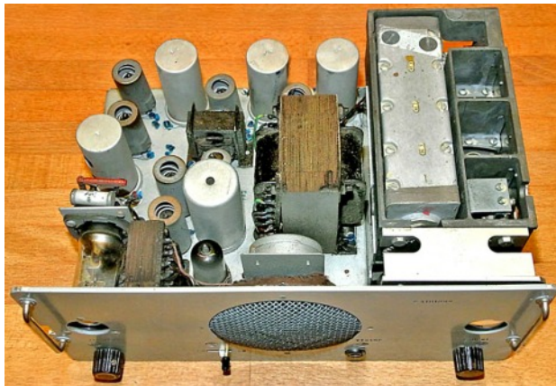
Top view of Sázava I chassis showing the Fug 17 front end unit (right) and IF strip (rear and left).
