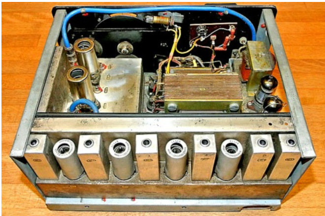
Top view of a Sázava II (TI-457) showing RF front end unit (top left with two valves on a silver plated enclosure); AC mains power supply and AF output stage (top right); IF strip (bottom).
