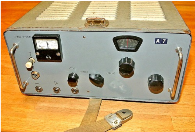
Front panel view of the Sázava II (TI-457). The tuning scale was not calibrated in frequency. A meter with a centre scale pointer allowed accurate tuning to the FM signal of a bug.
